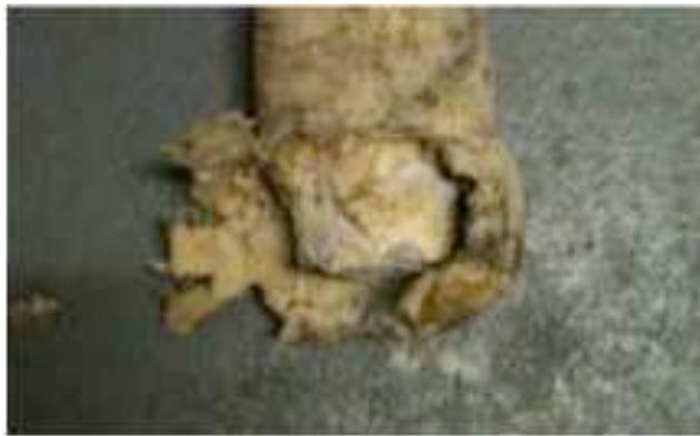
**Fig. 9 the magnesium anode was partially covered with a thick, well-adhered, scale.**
