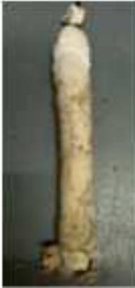
**Fig. 8 Magnesium anode after 6 months of service**
