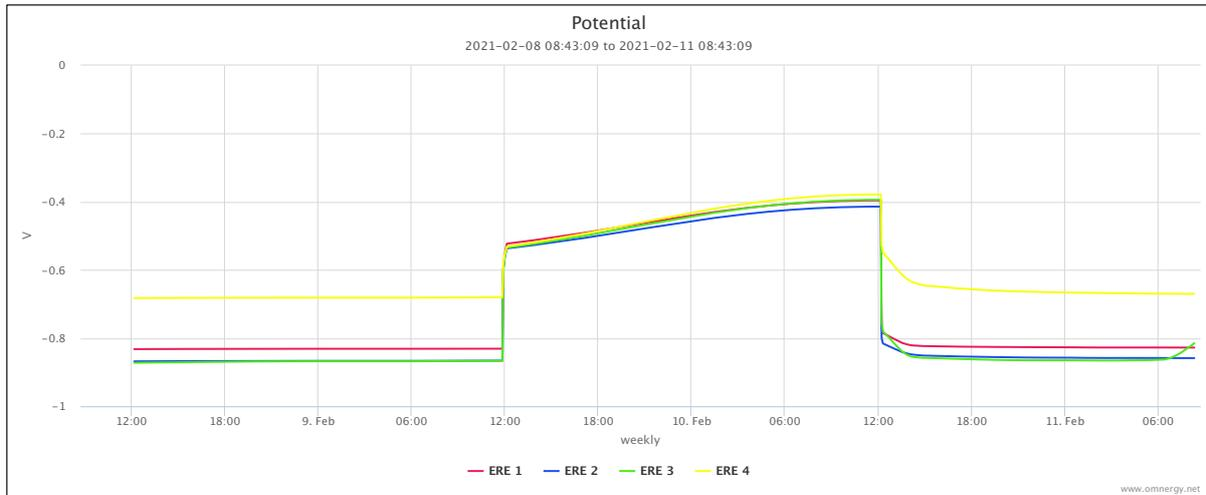
Fig. 16 Potential decay curves of zone 5 and zone 6
