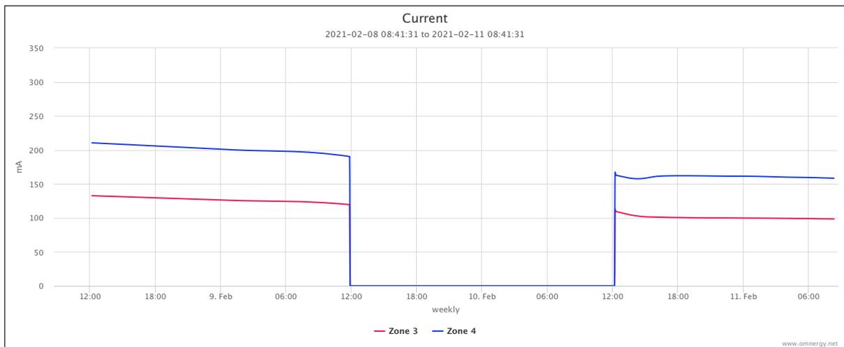
Fig. 13 GACP current output of zone 3 and zone 4 each appr. 53m<sup>2</sup> ZLA
