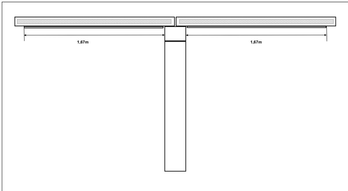
Fig. 6 ZLA applied up till 1,67m on both sides of the joint all along the joint.
