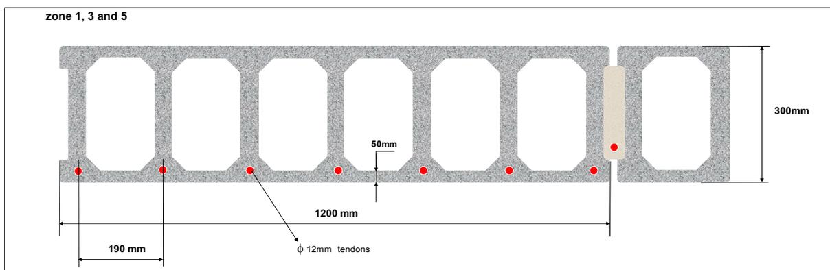
Fig. 3 Slabs located in zones 1, 3, and 5
