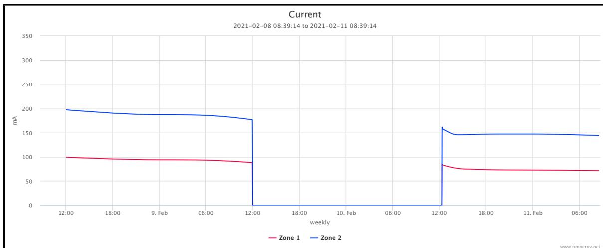
Fig. 9 GACP current output of zone 1 and zone 2 each appr. 53m<sup>2</sup> ZLA
