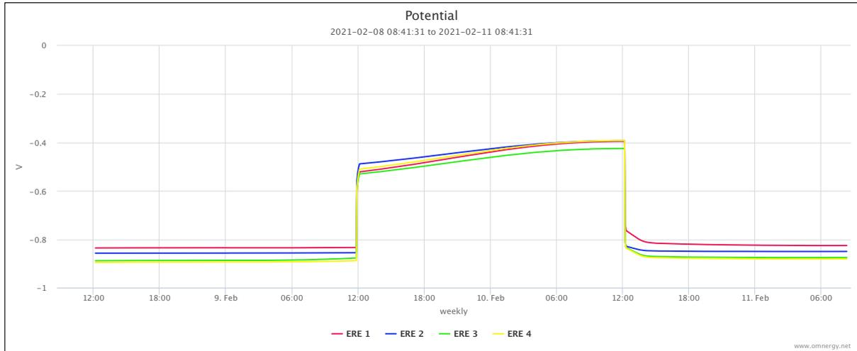
Fig. 12 Potential decay curves of zone 3 and zone 4
