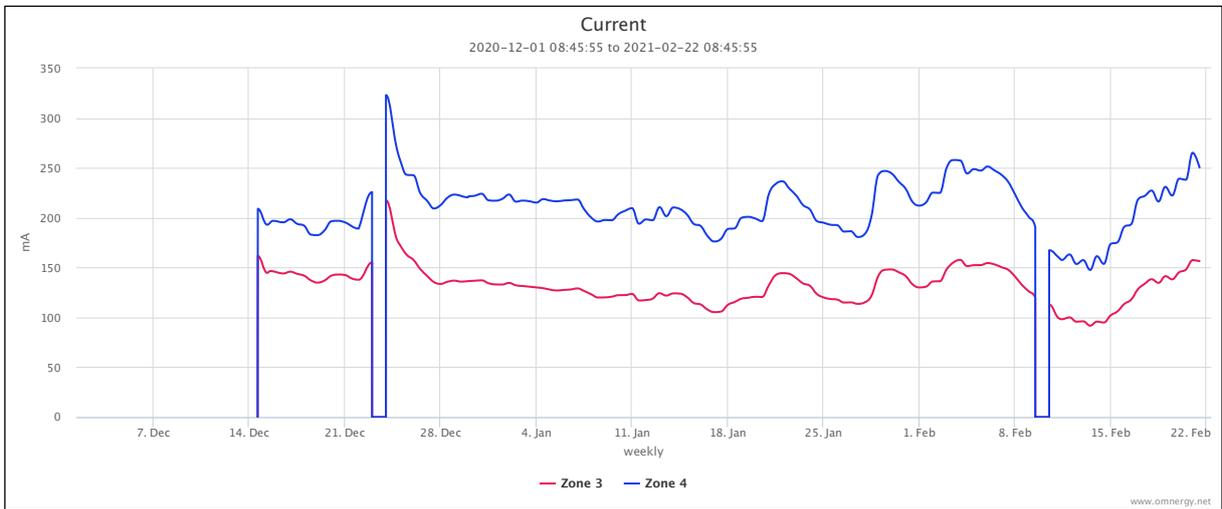
Fig.15 GACP current output since start-up of zone 3 and zone 4
