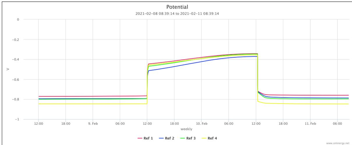
Fig. 8 Potential decay curves of zone 1 and zone 2
