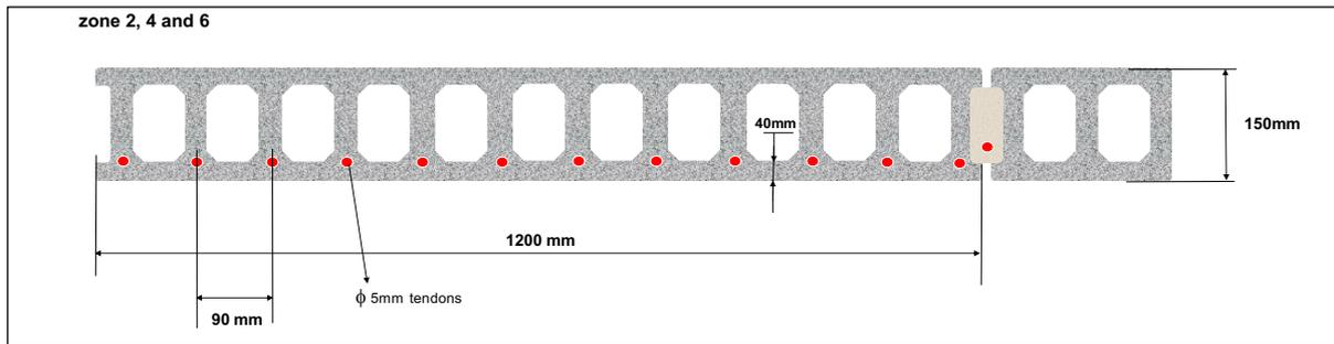
Fig 5 Slabs located in zones 2, 4 and 6
