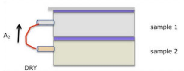
Figure 8. Electron flow of the macrocell condition
