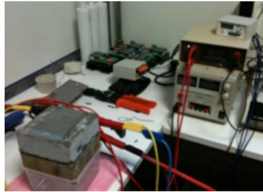
Figure 4. Lab set-up with two ZRAs measuring the current distribution and direction.
