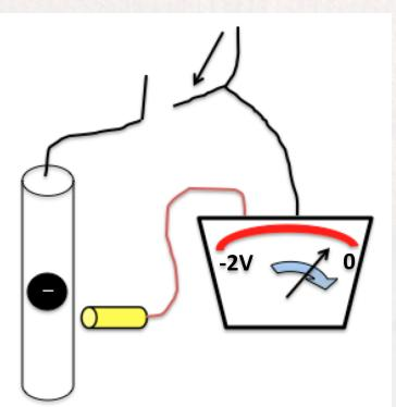
1. Charging the steel bar with millions and millions of negative particles will cause a situation in which I am pressurising the bar with these particles.
