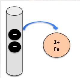
As can be seen the corrosion reaction charges the steel bar with negative particles, such as the current does.
