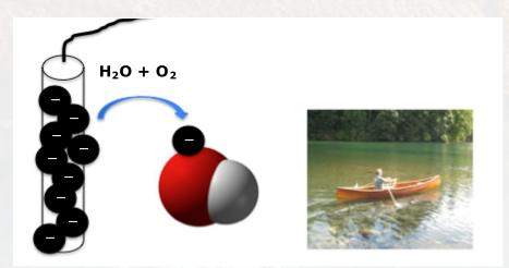
This process is an electrochemical reaction in which water and oxygen are consumed to form hydroxide-ions as electron carriers.
